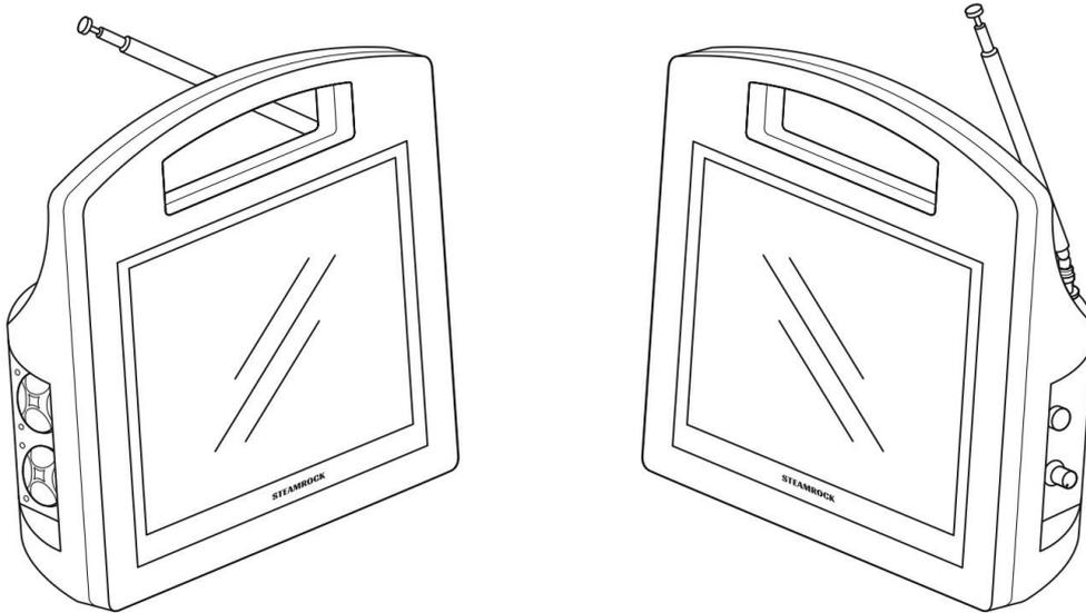
This device uses four alkaline D size batteries. The two battery compartments are located on the left side of the device. To insert the batteries, twist each cover counterclockwise a quarter turn and remove it. Put two batteries into each compartment **positive terminals pointing outwards**. Replace the covers.
