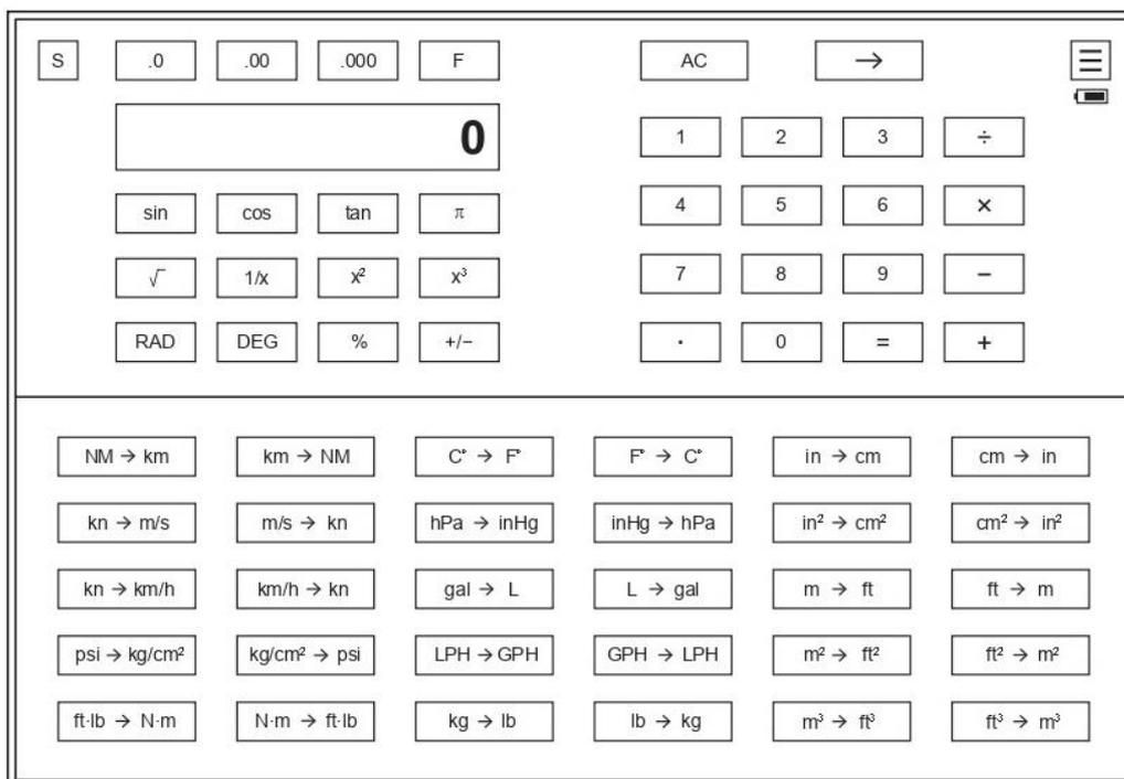
**The Math Screen** displays the calculator frame and the unit conversion operations frame.
