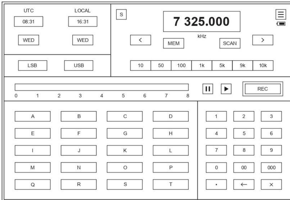
**HF SSB Receiver Screen** allows you to receive HF SSB voice broadcasts in LSB or USB mode within the 3 to 30 MHz range.
