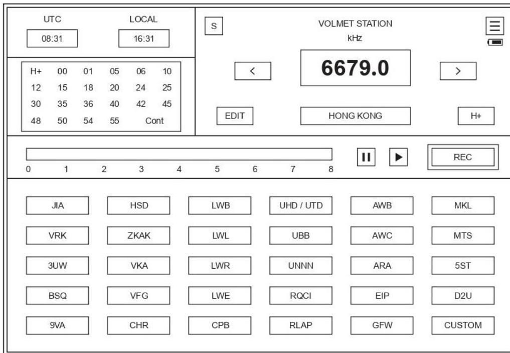
**The VOLMET Screen** gives you convenient access to international voice-broadcasted weather reports and forecasts for wide but relevant navigational areas. Although used for aviation, these broadcasts can be useful for mariners wanting a broad picture of the weather in a region.
