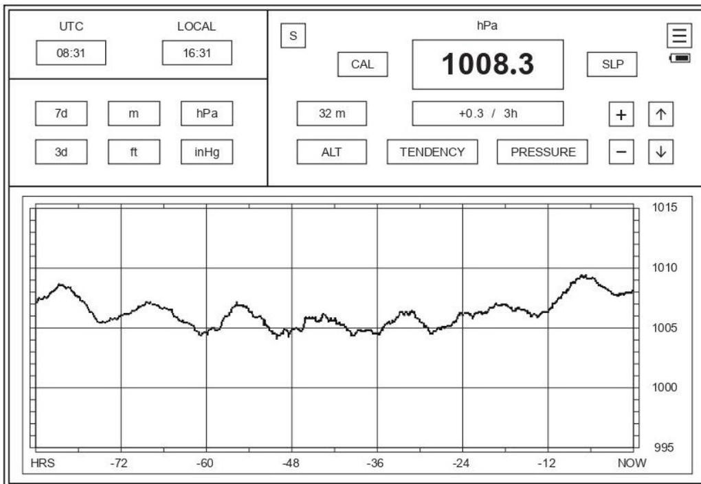
**The Barometer Screen** displays current atmospheric pressure and its changes up to 7 days. It has atmospheric pressure and tendency alarms that you can preset. These alarms keep you aware of significant weather changes whether or not you are using the Barometer function and even when the device is turned off.
